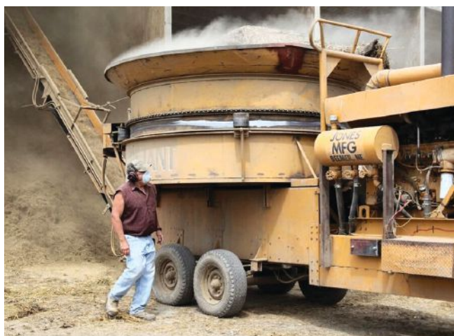
This worker is wearing hearing protection, a respirator, and a smart watch that monitors his heart rate.
