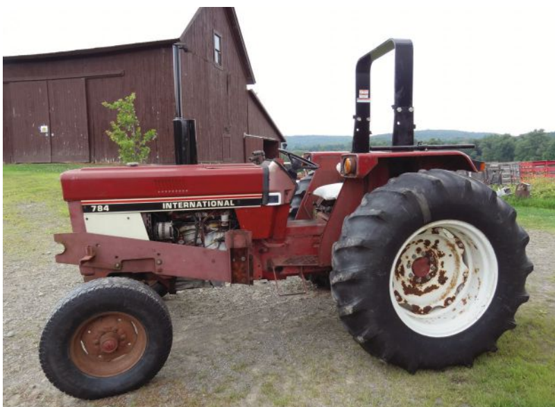
A typical ROPS retrofit from the National ROPS Rebate Program.
