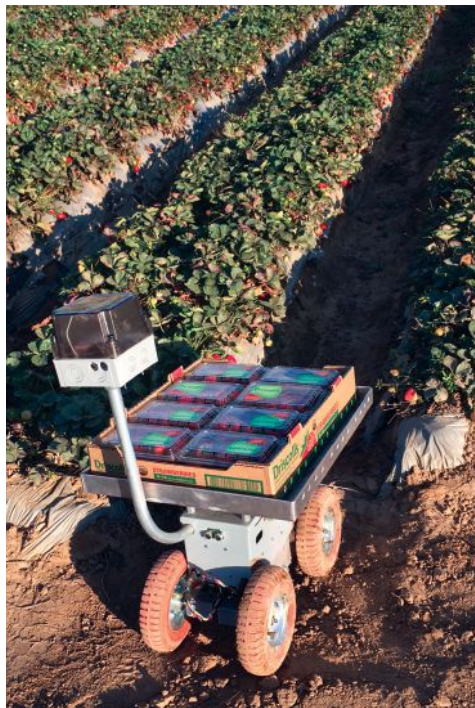
A collaborative robot that assists workers in transporting strawberries during harvest. Photo courtesy of Stavros Vougioukas, University of California-Davis.
