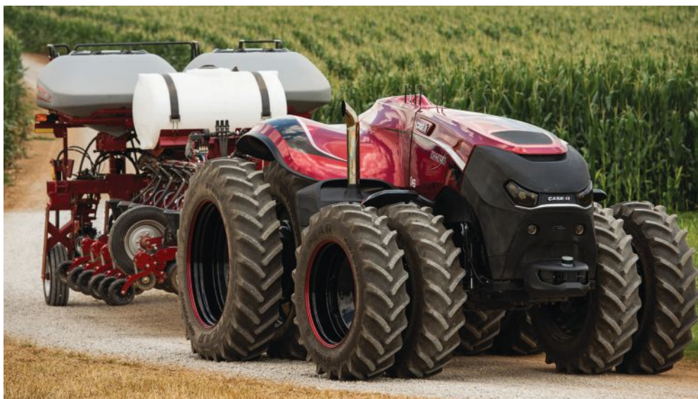
Autonomous field machines have potential to revolutionize agricultural production, but safety concerns must be addressed before widespread implementation. Photo of Magnum autonomous concept tractor with model 2150 planter in transport courtesy of CNHi.
