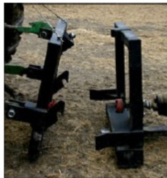
Backing Tractor to Implement
