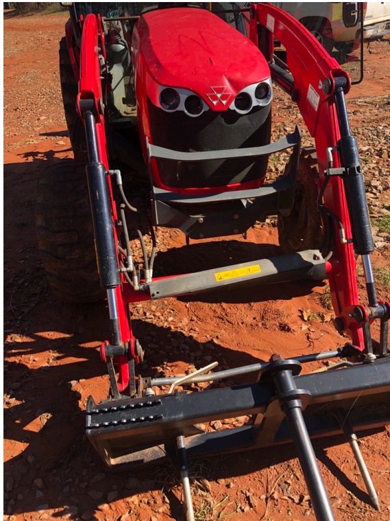
Skid Steer Style Connection
