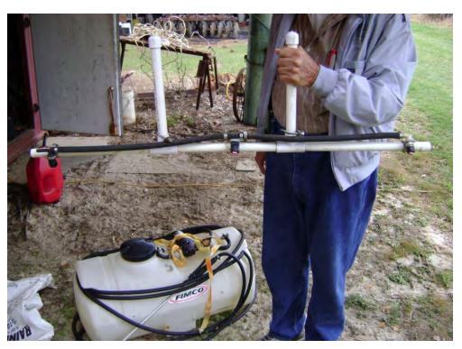
The farmer has a sprayer that only has the handheld wand sprayer. He made a boom for the sprayer that allows him to attach it to the back of his UTV and spray a wider area. The boom is made out of PVC pipe and fittings. The hose with the spray nozzles is attached to the PVC using U-bolts.
