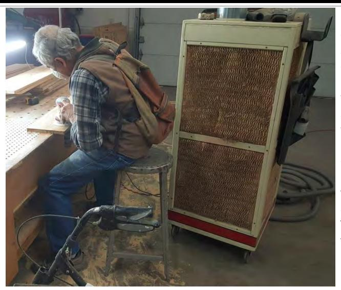
Don has muscular dystrophy so his torso slumps forward. He figured out that wearing a backpack with 11 pounds of weight in it helps hold his shoulders back while he is working in his farm shop. He also built an air cleaner cabinet with a shop vac inside and furnace filters on the sides to control dust and improve his breathing. The shop vac draws air through the filter and blows clean air out the duct in top of the cabinet.
