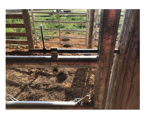
The farmer made a springloaded gate latch using a gate hinge, a piece of rebar, spring, and a bolt. The latch allows the farmer to quickly go into the feeding area without having to wrap and unwrap the chain.
