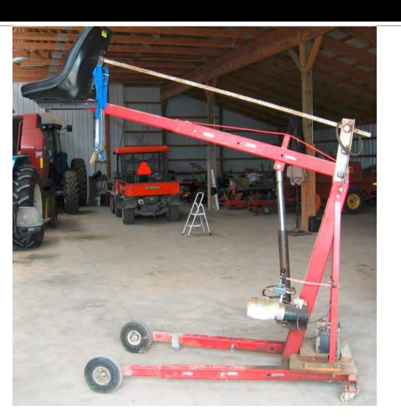
Jerry modified an engine hoist to lift him into his tractors. He used a 12V hydraulic power unit and hydraulic cylinder. A bucket seat with seatbelts pivots on the end of the hoist with a parallel linkage so it remains level as he raises up. A helper rolls the hoist near to the tractor so Jerry can make the transfer.
