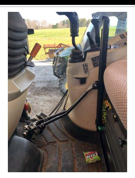
The farmer made his own hand controls for his hydrostatic tractor. The control levers are made out of standard pipe and are hinged at the bottom. To connect the pipe to the hydrostatic pedals, the farmer used shift rod linkages that can be bought off of Amazon. He bent the shift rod linkages to get the angles needed for the hand controls.
