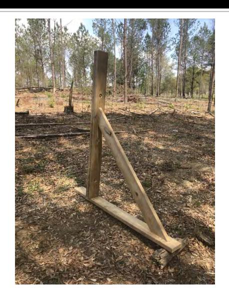
When installing long runs of fencing, the fence would bend in the middle. The farmer built a holder out of wood. Two 2x6s bolt together to keep the fence from bending. The base rests on top of the ground and slides as the fence is tightened by the stretcher.
