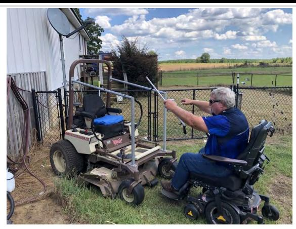
In order to get back on his lawnmower, the farmer fabricated grab bars out of square tubing and pipe. He bolted the grab bars to the ROPS and frame of the zero-turn lawnmower. He can pull himself up with the bars and they help to improve balance while standing.
