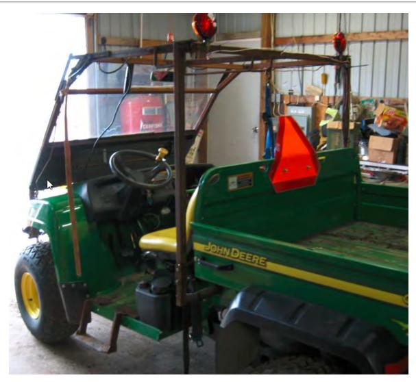
Steel frame concocted to provide grab bars for transfers and a step up to the vehicle deck.
