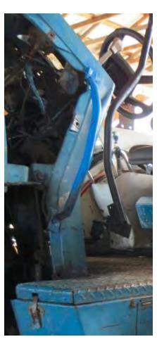
A grab bar as shown below can be simply made by flattening the end of a pipe, bending it in a 'u' shape, and drilling holes in the flat to match your tractor bolt holes (and orange paint!).
