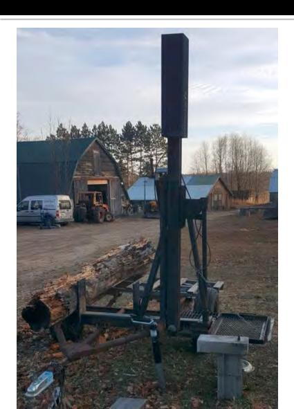
Bob mounted this Life Essentials manlift platform on a trailer that he can move around with his Kawasaki Mule. He can park it close to the tractor, walk from the Mule to the manlift, and raise himself up to the operator station. A fold-down 'bridge' was added so he can walk safely from the platform to the tractor seat without stepping over gaps.
