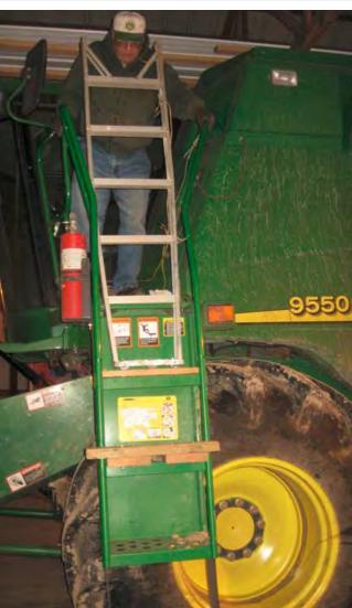
Joe hinged a lightweight ladder to his combine, so he has sloped steps closer together. He flips the ladder up with a rope while driving.
