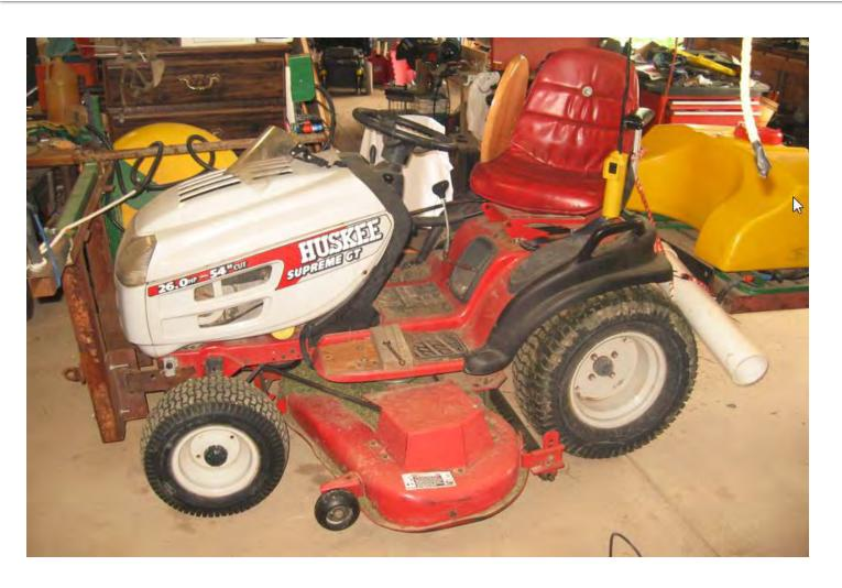
A swivel seat from a fishing boat has been installed on a lawn tractor. David outfitted this tractor with a sprayer and chemical tank so he can control weeds in his blueberry fields. A wood panel provides posture support.
