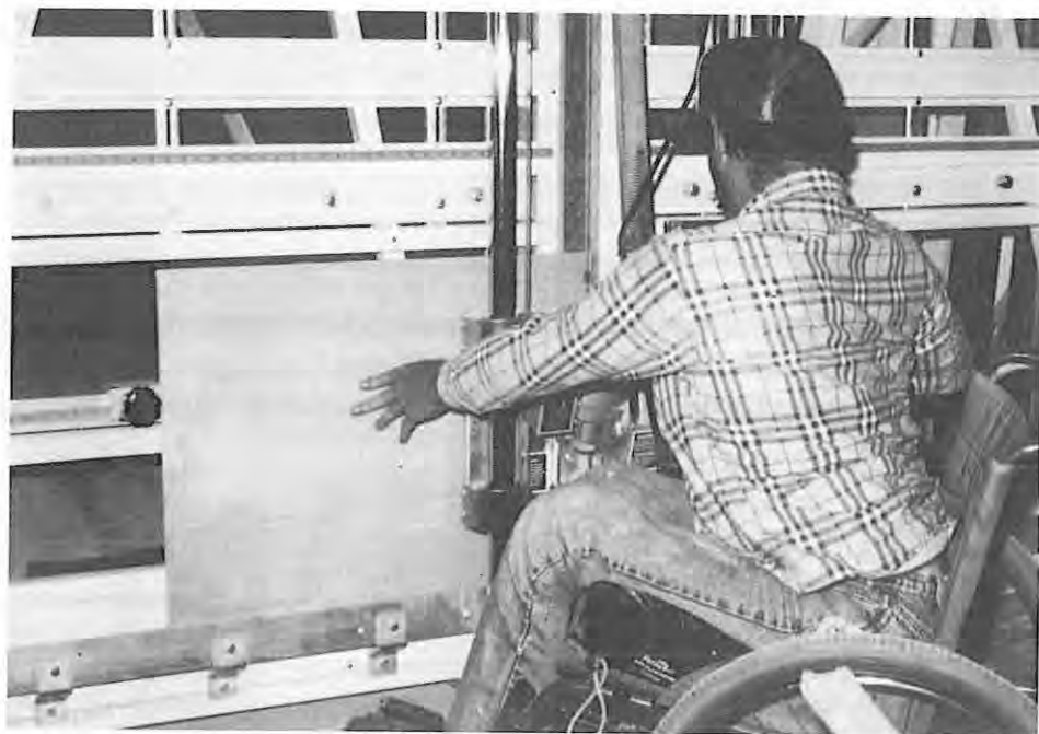
This vertical table saw is somewhat more accessible than Kurt's standard table saw, particularly when handling larger sheets of ply-board and other heavy lumber.
