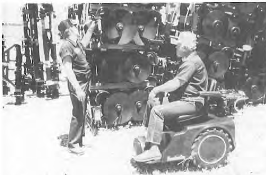
Arlan utilizes a Freedom-I all-terrain, motorized wheelchair for mobility around the shop and yard. The three-wheeled chair is equipped with electric and gasoline motors, as well as a powerful hydrostatic drive transmission.
