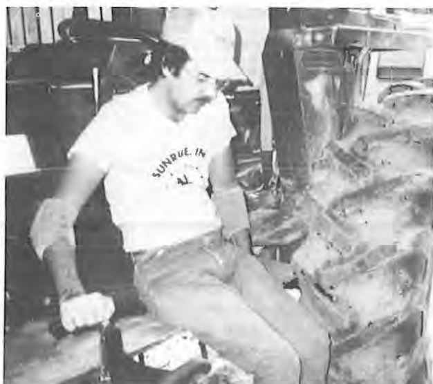
Ed modified his tractors by installing high-back seats, seat belts and hand controls. His other tractor includes a lift.
