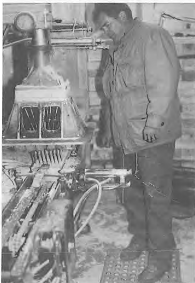
Ron uses a special press to drill his "bee boards." Bees lay eggs in each hole then include nectar for the larvae's nourishment and cap the hole with a piece of alfalfa leaf.
