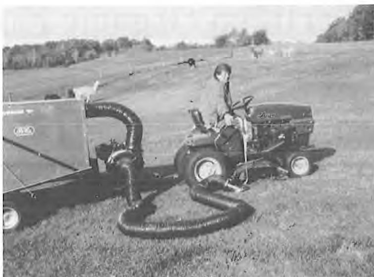
Judy markets llama manure as high-quality fertilizer. The manure is collected with a "Pasture Vacuum" pulled by a lawn and garden tractor.
