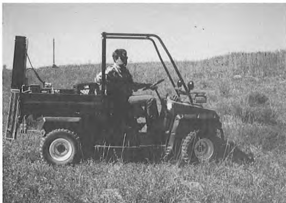
Chris' consulting firm, Soil Systems, utilizes a Kawasaki Mule 4-wheel utility vehicle specially modified to carry a hydraulic core sampler (bottom, facing page) and soil data recording equipment (top, facing page).
