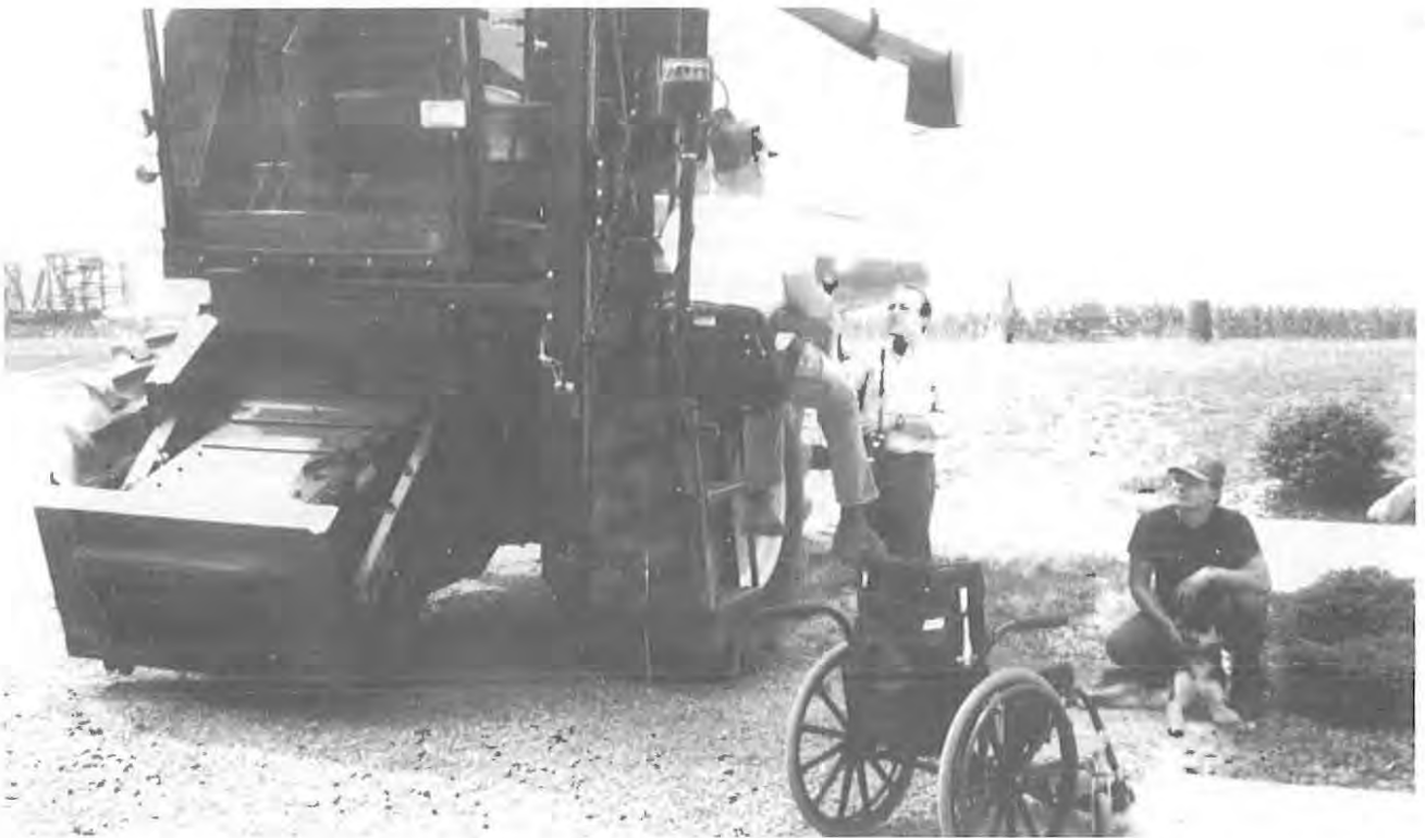
Arlan modified his IH 1460 combine with a man-lift to provide access from his chair to the operator's seat. The independently controlled lift operates by a vertical-screw mechanism, and receives power from the combine's battery.
