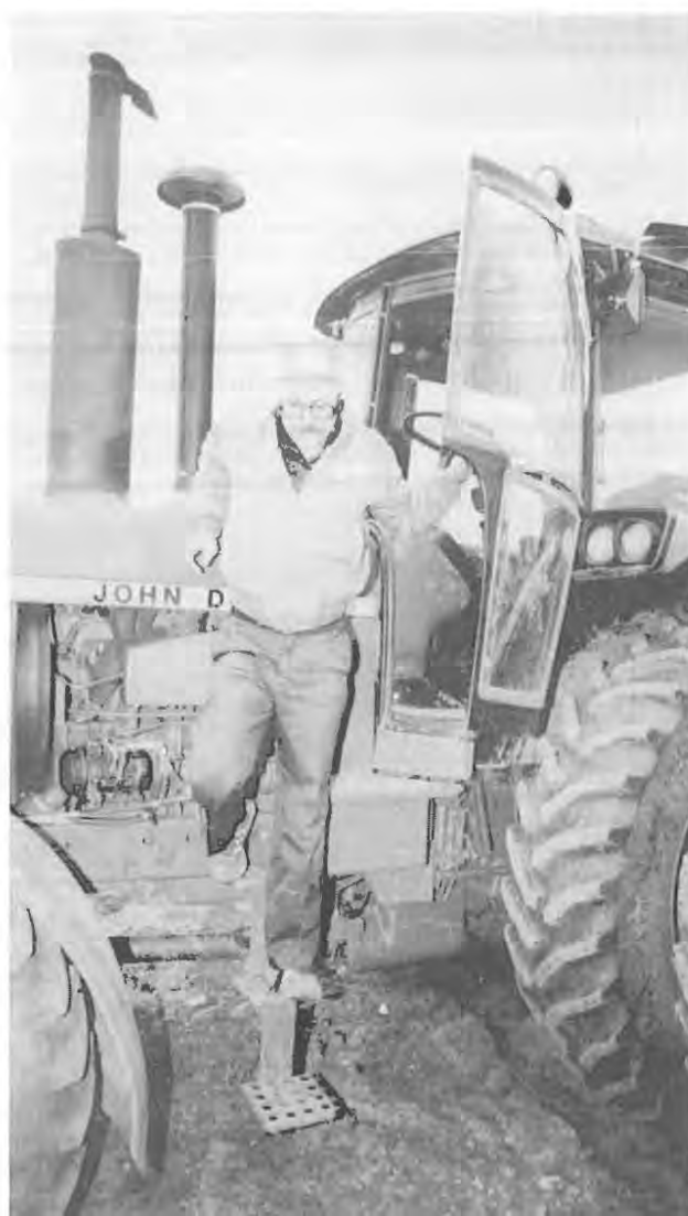
Dan equipped his tractor with extra steps to provide easier access to the tractor cab and seat.
