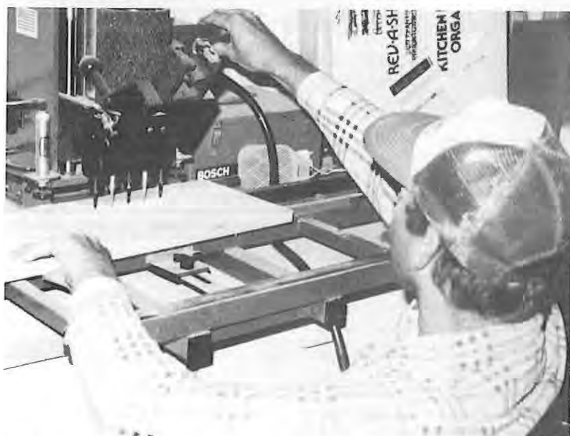
This drill-press and other machines in Kurt's shop were made more accessible by cutting out a space in the cabinet to allow clearance for his chair.
