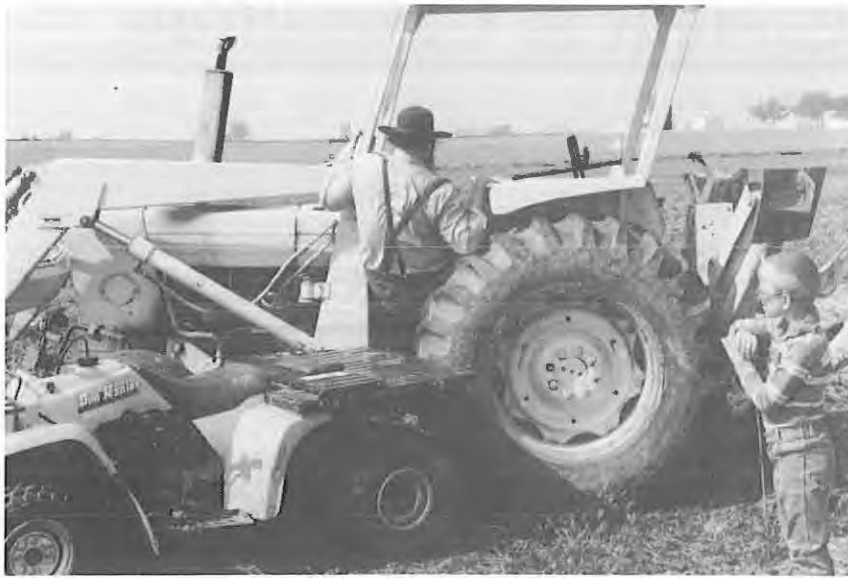
Carl is able to access both his ditcher and backhoe by pulling alongside on his 4-wheeler, sliding across the bed, and pulling himself into the seat. The foot shifter on Carl's Yamaha 4-wheeler was replaced with a hand-control shifter.
