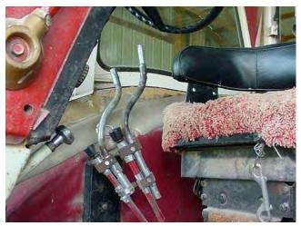
Picture 3. Extended and bent control levers.
