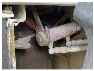
Picture 2. Auxiliary hydraulic clutch.
