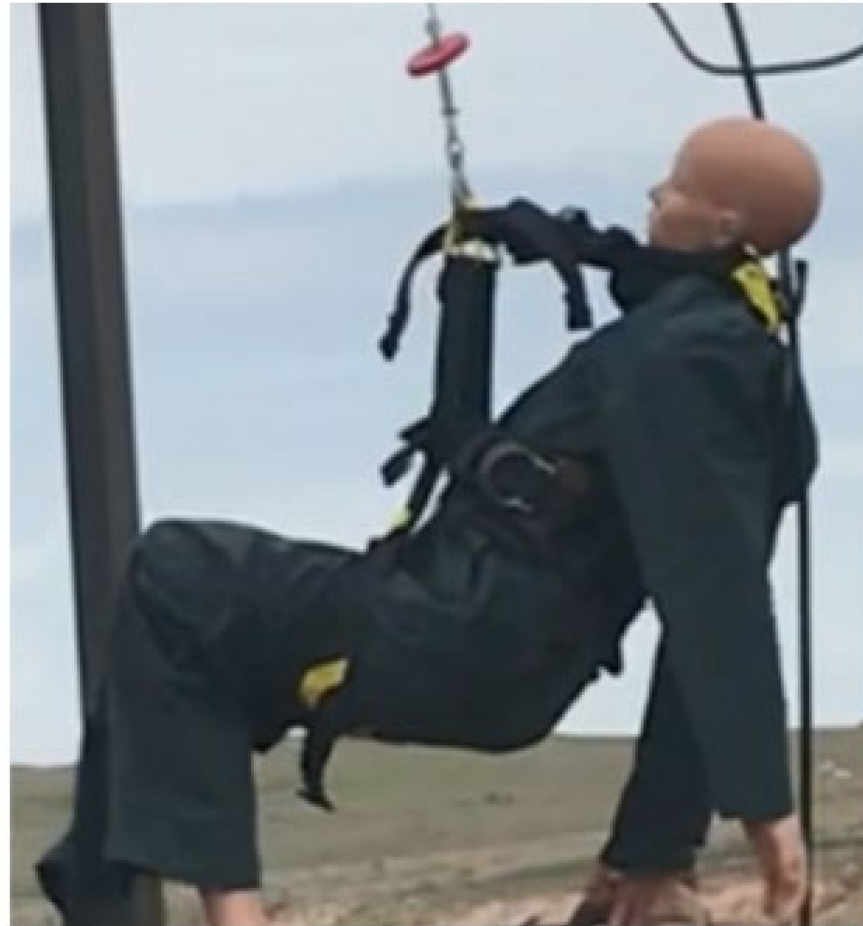
Figure 43: Petzl Volt harness keeping dummy in a seated position
