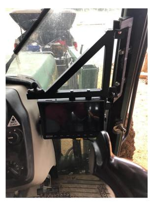
Agricultural cameras were added to his tractor to give him a view of the back of the tractor and the front-end loader. The camera in the back includes digital guidance lines to make it easier to hook up to equipment. The cameras also allow him to see the implement while using it without turning around and looking. This has helped to reduce dizziness when looking forward and backward.
