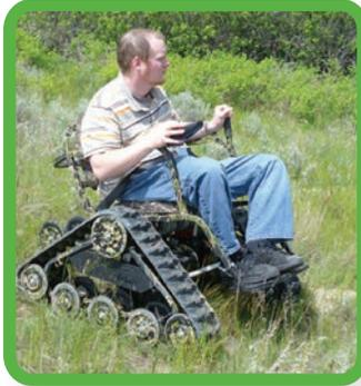
The joystick-operated **Action TrackChair** runs off two 12-volt batteries that feed its 24:1-ratio high-thrust motor. It reportedly has a 5-mph top speed, an 8-mile range, a zero turning radius, and 200-pound load capacity. Standard features include 23-inch-wide seat with 20° tilt, adjustable foot rest, and six accessory holders. Visit [www.actiontrackchair.com](http://www.actiontrackchair.com).
