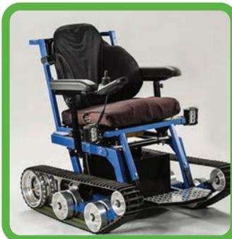
In addition to its outdoor-navigation capabilities (e.g., snow, mud, sand, gravel, grass, even curbs), the joystick-steered **TrackMaster Power Chair** is also designed to be used indoors because of its narrow width (only 29 inches) and its omni-wheel retractable-tracks system, which reportedly won't damage flooring. Visit [www.track2freedom.com](http://www.track2freedom.com).
