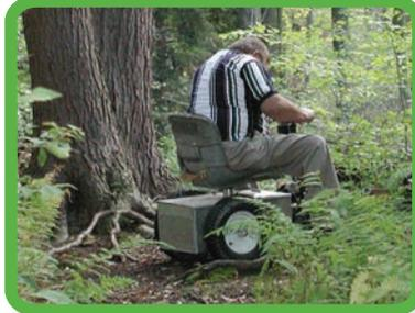
Powered by two 12-volt gel batteries that drive its four motors, the **Journeyman Scooter** is designed to climb hills, cover rough terrain, and wade through up to 6 inches of water without danger of hanging up, tipping over, or stalling out. It features front suspension, large tires, rust-resistant aluminum body, and 4-inch ground clearance. Visit [www.lifeessentiallifts.com](http://www.lifeessentiallifts.com).
