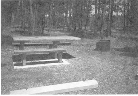
Figure 13: This accessible campsite displays the swing-away fire ring grill, the cut-off picnic table bench and the smooth, flat ground cover.
