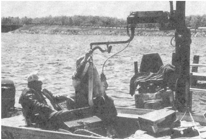
Figure 19: Lifts may also be used by fishermen with disabilities to access their fishing boats without using ramps.
