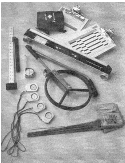
Figure 16: Simple tools are used to measure grade, cross slope, width and other characteristics of trails. The tool kit is available through Beneficial Designs 16 for those interested in evaluating trail accessibility.
