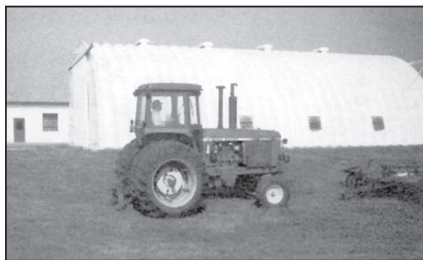
Figure 2: The tractor cab is an example of isolating a person from a noise source.
