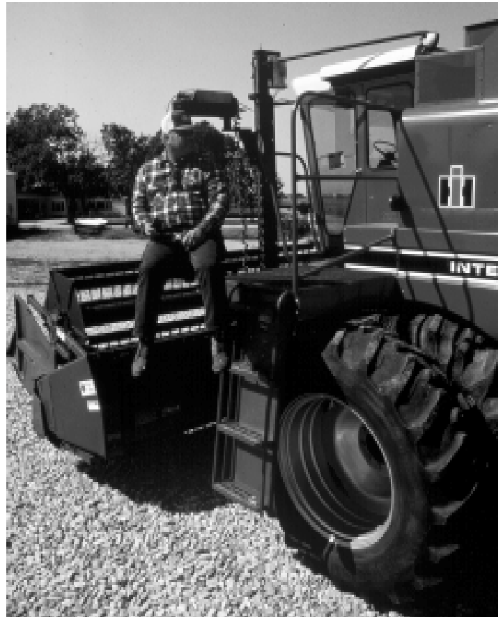
Figure 9. A vertical mast chair lift mounted on a large combine
