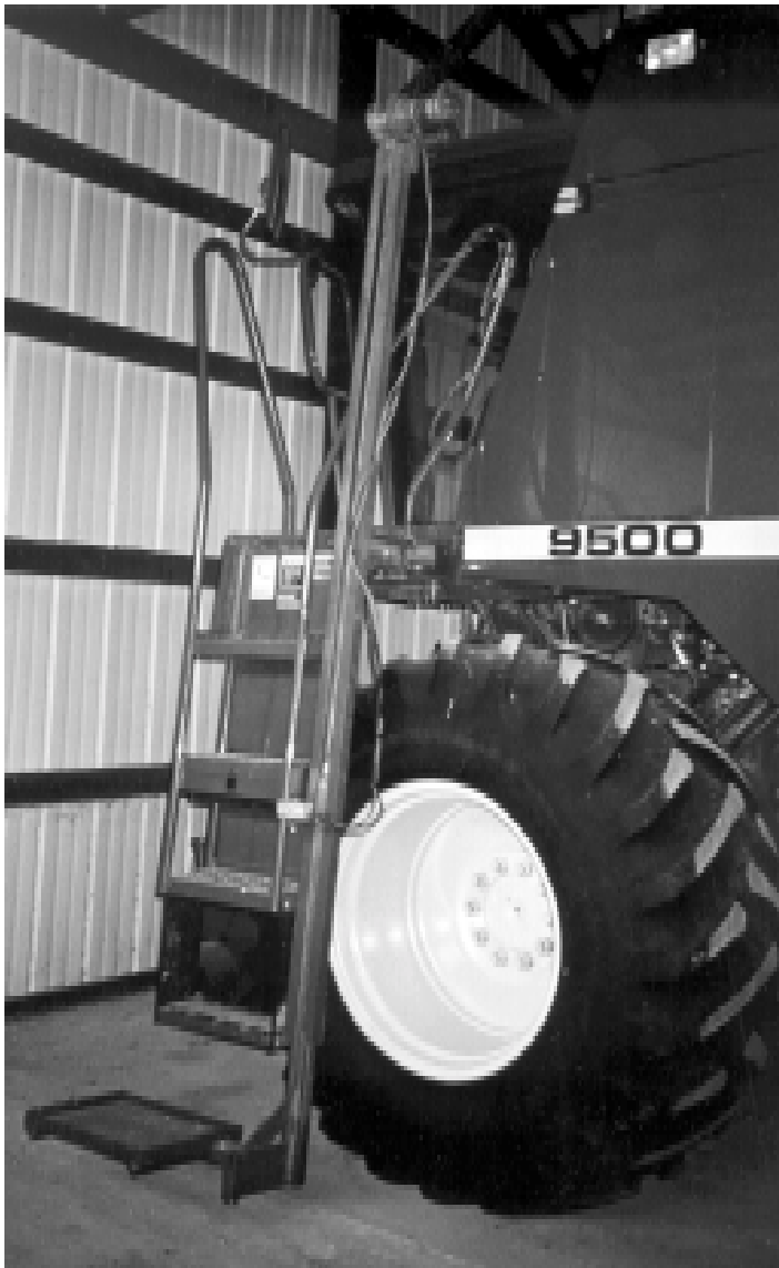
Figure 18. Dick Welty's winch-operated platform lift on his John Deere 9500 combine.
