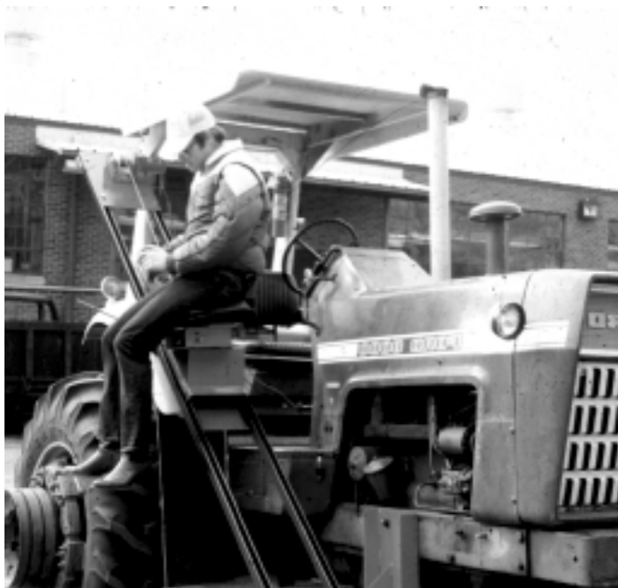
Figure 2. Prototype winch-powered access lift from the early 1980s.
