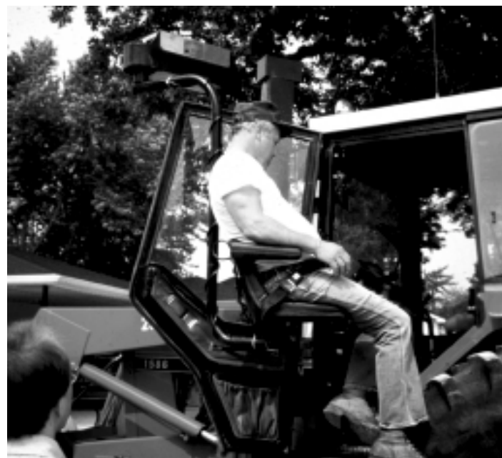
Figure 11. A vertical mast chair lift used with a front-mounted cab door.
