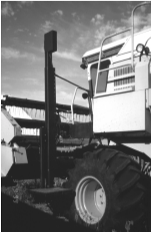
Figure 8. A vertical mast platform lift on a combine.
