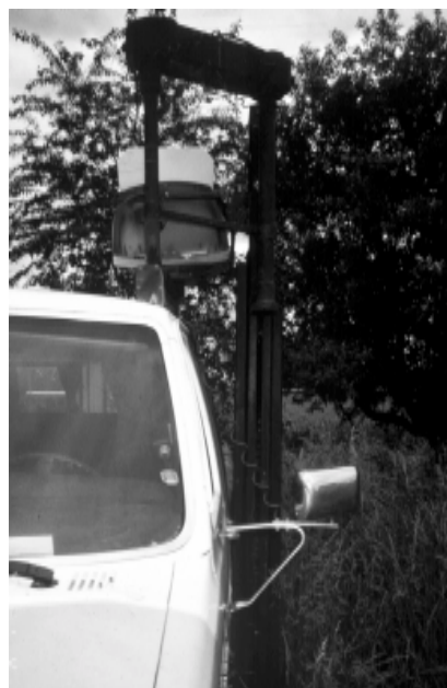
Figure 17. Bob Yeagle's vertical mast chair lift mounted to his van.
