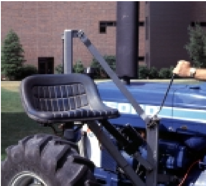
Figure 6. A parallel linkage lift mounted on a Ford 4610 tractor.
