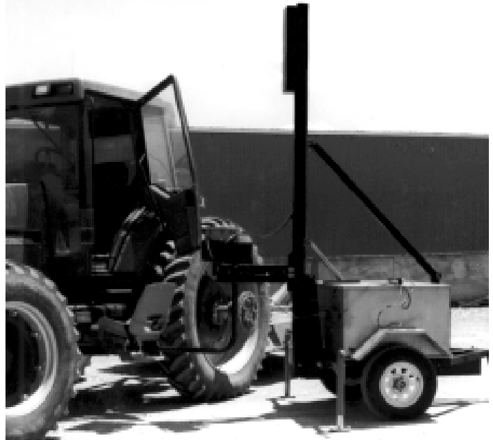
Figure 14. An independent lift mounted to a trailer that can be towed anywhere for access to machinery.
