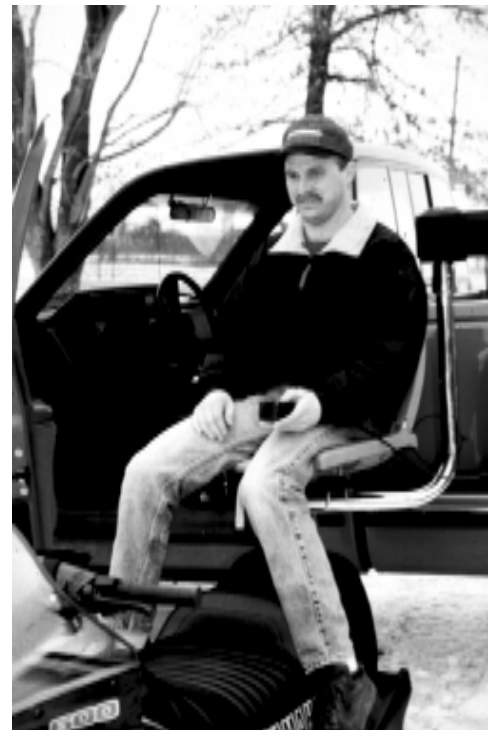
Figure 5. An independent lift mounted on a pickup truck.
