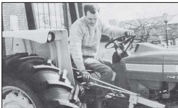
Figure 7. Hand brakes mounted on a small farm tractor. An over-center mechanism is incorporated to allow the operator to lock the brakes.
