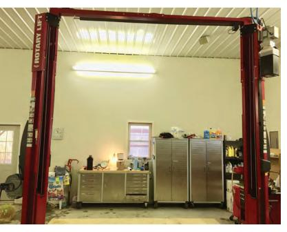
Figure 4. Wall-mounted lighting provides both top-down reflected light and side-angled light, resulting in less perceived shadows on work areas.
