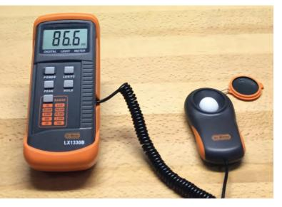
Figure 1. Digital light meter used to measure available light in work area.
