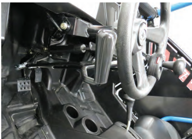
Figure 4. Modified UTV foot controls using horizontal lever connected to the pedals with adjustable mechanical linkages. (Source: SureGrip HVL)
