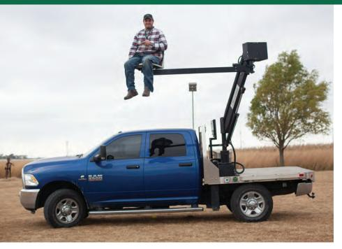
Figure 7: Pickup truck-mounted independent access lift.
