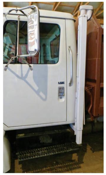
Figure 13. Ball-screw drive sideboard access lift mounted on a grain truck.
