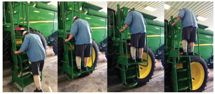
Figure 4. Platform lift with fold-away platform allows easy entry for both users in need of assistance and able-bodied users.
