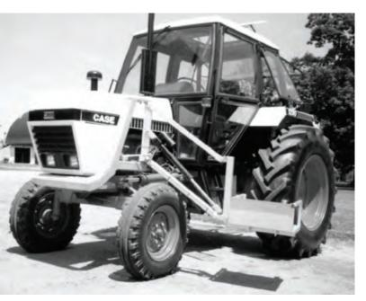
Figure 1. 1980's access lift concept, BNG Mark II man-lift.
