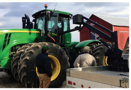
Figure 9. Independent access lift allows user to access locations up to 12 ft. up and 14 ft. away from the host vehicle.
