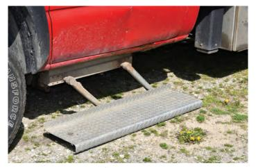
*Figure 5. Running board lift to assist driver (and/or passenger) into vehicle.*
