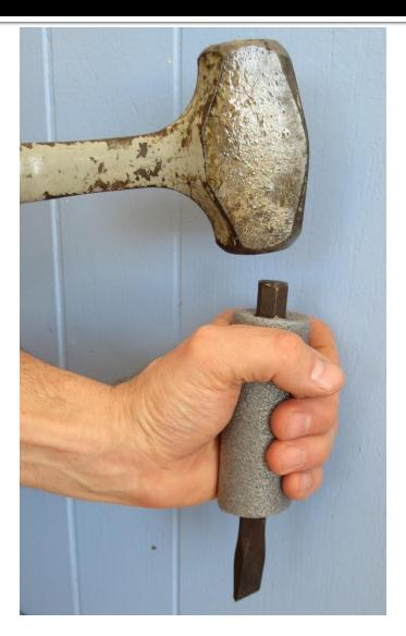
Small-diameter handles are especially difficult to hold securely when a person has hand injury or disease. Increasing the diameter of a tool handle and making it soft allows the worker to hold it tightly with less grip force of the hand. Fabric strips, foam padding or any other cushion material can be wrapped around small tool handles. Hand tools used with high-force should have 1 <sup>3</sup>/<sub>4</sub>" diameter handles for maximum grip strength.
