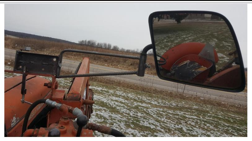
This extension mirror is constructed of a welded steel rebar frame and a mirror from a scrap Ford van. Ford vans have very good mirrors for this. The extension is 15-inches long and can be clamped or bolted onto tractor fenders or frame. The mirror helps workers with neck injuries see behind the tractor.
