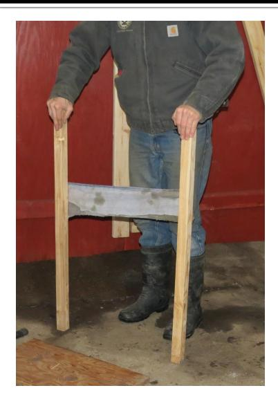
This back-support frame is a strap of cloth fastened between two wooden poles. The strap is 18-inches long and 4-inches wide. It supports the upper body and takes the pressure off the lower back when reaching forward in a kneeling or stooped position.
