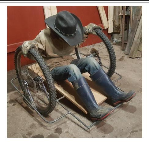
Scrap wheels cut from bicycles welded to a steel rebar frame. The platform is 22-inches wide and 42-inches long. The platform is suspended 3-inches above the ground and balances between the two wheels. The foot end of the platform lightly drags on the ground. The low platform is convenient to slide on and off from ground level.
