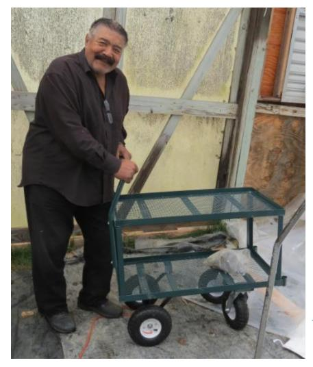
A Walker Cart enables workers to carry loads around the farm and lean on the cart for balance at the same time. This walker cart can also be modified with a lowered seat cushion on the cart to sit and 'pull' along as needed. Produce, plants and small loads of other materials are often picked up and moved. Carrying such loads is impossible to do with poor balance. These materials can be loaded onto the cart and then pushed to the destination with much less effort than carrying.
