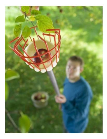
Workers who cannot climb can pick fruit from the ground. The Pole-Mounted Fruit Picker is a wire basket at the end of an 8foot pole, with wire fingers protruding out from the top of the basket. The fingers hook around the fruit and pull it into the basket, which the user then lowers to the ground and empties.
