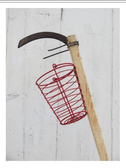
Any type of small basket or pail mounted to the end of a pole will catch falling fruit. A blade for cutting stems or prongs for plucking fruit from the branch can be fasted with nails, screws, or straps.
