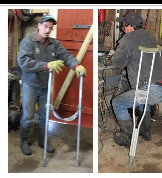
One end of a fabric strap is sewed onto a crutch, and the other end sewed onto a hook. When ready to sit down for a rest, the strap is hooked across the two crutches to form a seat. When walking, the strap is hooked to one crutch. The 18-inch long strap is 3-inches wide and made of scrap denim from old clothing.
