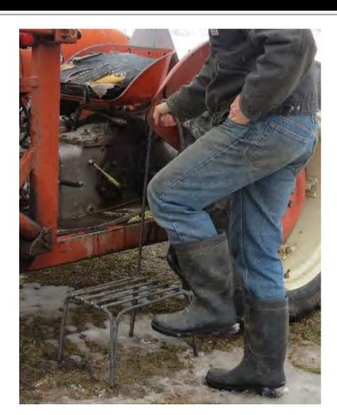
This step stool with grab handle is constructed of welded steel rebar. It is 15-inches long, 10-inches wide, and 10-inches tall. It helps farm workers with leg impairments climbing up to reach items on a high shelf, or climbing up steps on equipment.
