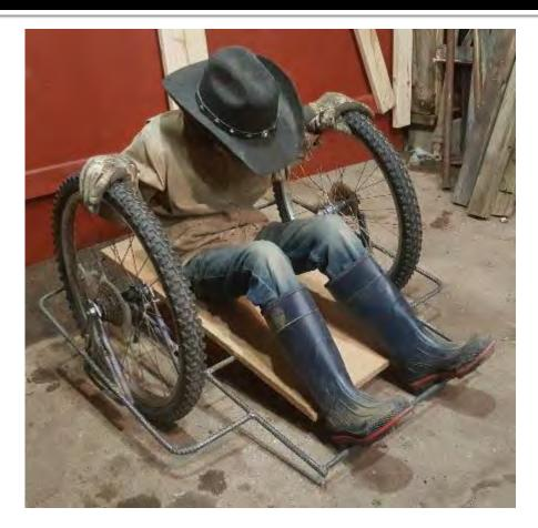
Scrap wheels cut from bicycles welded to a steel rebar frame. The platform is 22-inches wide and 42-inches long. The platform is suspended 3-inches above the ground and balances between the two wheels. The foot end of the platform lightly drags on the ground. The low platform is convenient to slide on and off from ground level.
