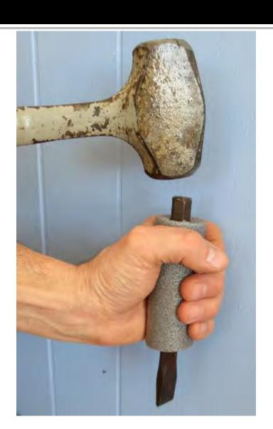
Small-diameter handles are especially difficult to hold securely when a person has hand injury or disease. Increasing the diameter of a tool handle and making it soft allows the worker to hold it tightly with less grip force of the hand. Fabric strips, foam padding or any other cushion material can be wrapped around small tool handles. Hand tools used with high-force should have 1 3/4" diameter handles for maximum grip strength.
