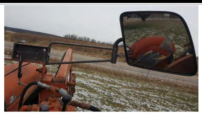
This extension mirror is constructed of a welded steel rebar frame and a mirror from a scrap Ford van. Ford vans have very good mirrors for this. The extension is 15-inches long and can be clamped or bolted onto tractor fenders or frame. The mirror helps workers with neck injuries see behind the tractor.
