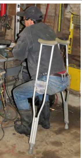
One end of a fabric strap is sewed onto a crutch, and the other end sewed onto a hook. When ready to sit down for a rest, the strap is hooked across the two crutches to form a seat. When walking, the strap is hooked to one crutch. The 18-inch long strap is 3-inches wide and made of scrap denim from old clothing.
