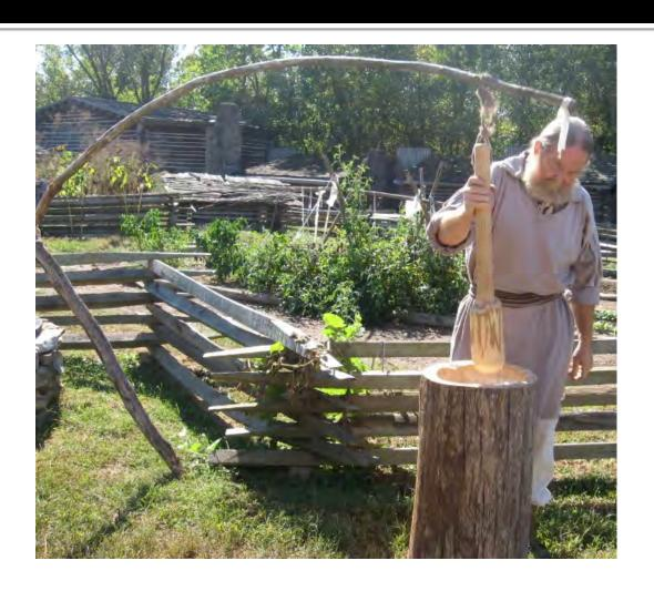
A tool balancer holds the weight of a tool for a worker with back and arm impairments. The worker can move the tool easily without the burden of holding it up. A tree branch can serve as a readily available tool balancer when the task can be positioned in an appropriate place.
