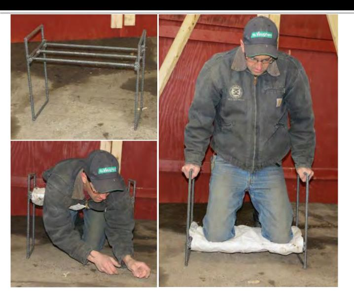
Kneeler seat and back support fabricated from steel rebar, widely available material around the world. It is 23-inches wide, 19-inches tall, and 10-inches deep. The kneeler platform is 4inches above the ground.
