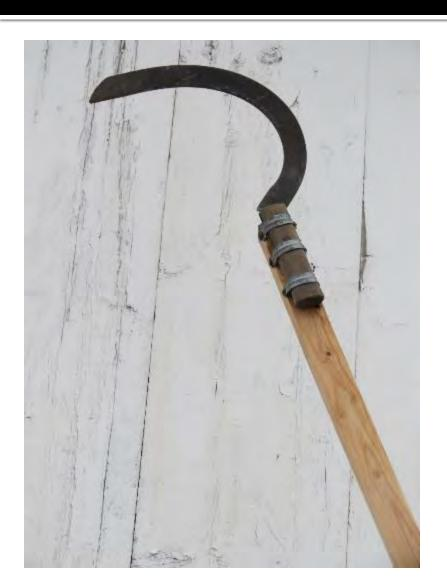
This sickle is fastened to a pole with this strips of scrap steel. Pruning trees can be done without climbing ladders.
