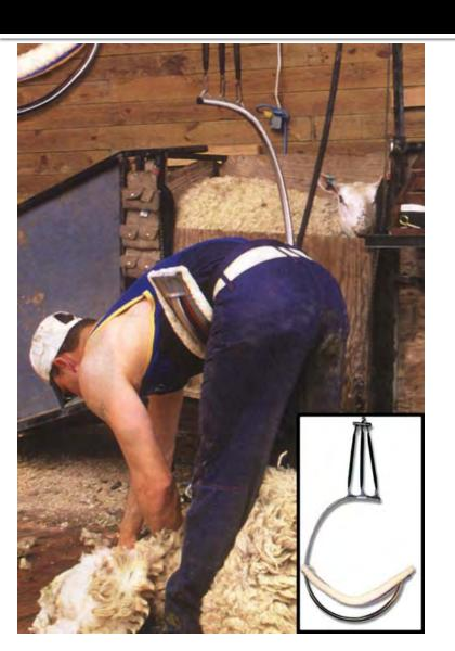
A Crutching Frame with Chest Belt can help reduce back fatigue while shearing sheep. The device is a steel loop with a padded chest belt across the bottom on which the shearer rests his upper body while bending over to shear sheep. The frame hangs from a beam by spring-loaded cables, which balance the weight of the shearer to take the pressure off his/her back.
