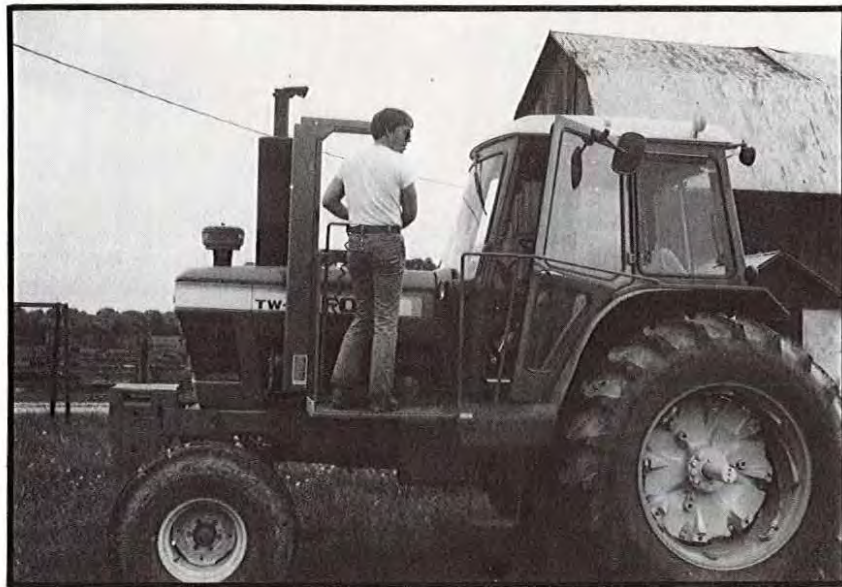
Figure 10. Operator Moving Onto Cab Entry Platform
