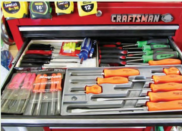
Identify contents of storage cabinets/containers with plastic backed, high contrast labels.
