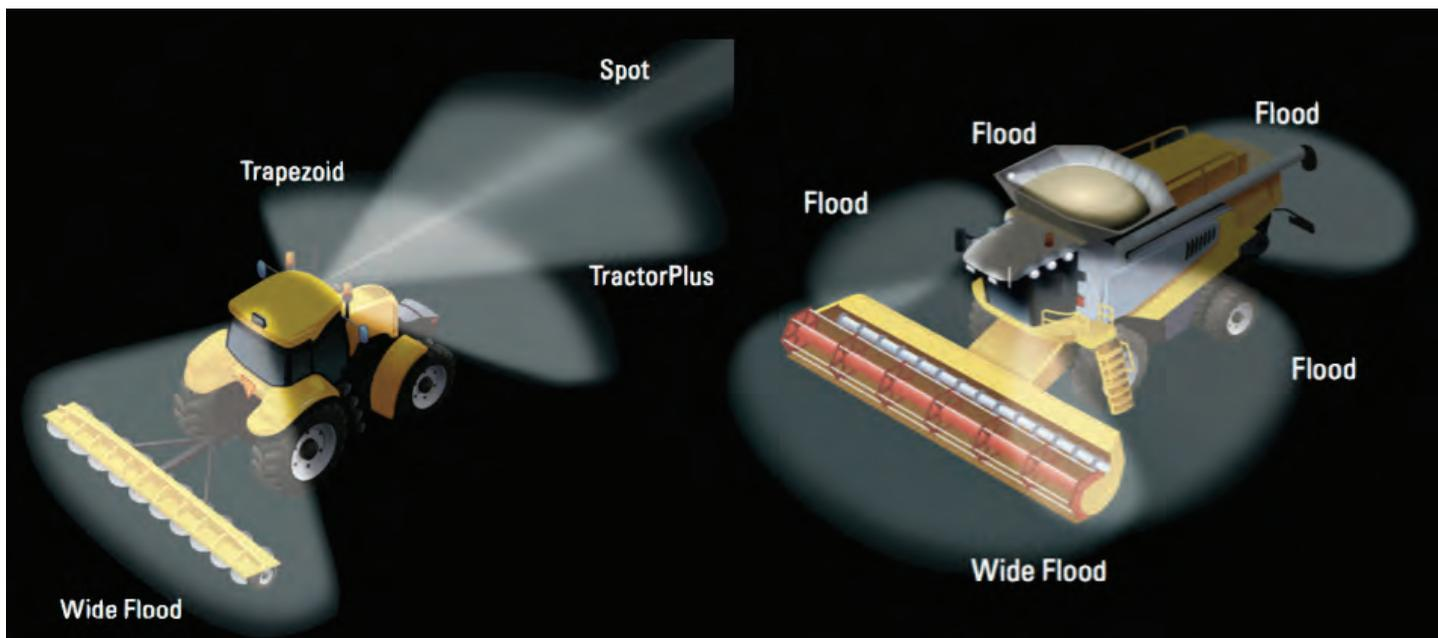
Figure 7. Light type and placement on self-propelled agricultural machinery. (Source: Modified from Grote 2016)
