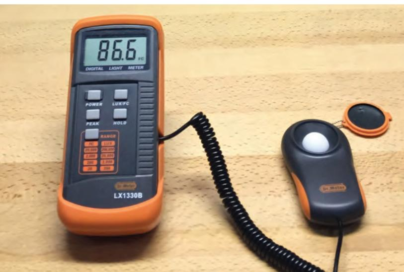
Figure 1. Digital light meter used to measure available light in work area.
