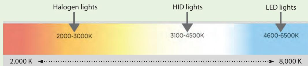
*Figure 3. Color temperature (Kelvin) affects the light appearance on illuminated objects and varies by light type/source.* (Source: Deere and Company, 2010)
