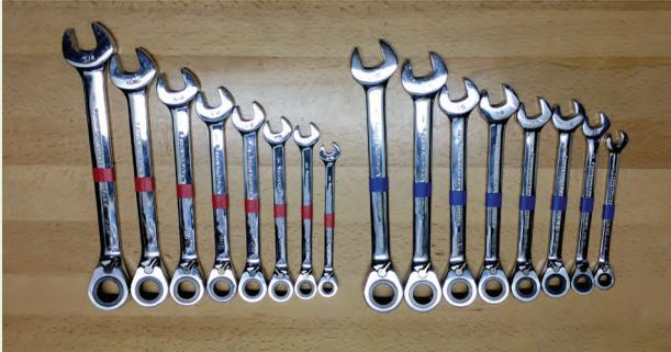
Purchase laser-etched size labeled sockets and wrenches for easier reading.
