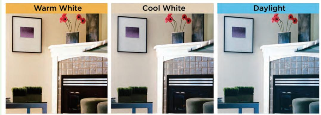
*Figure 2. Changing color temperature of light affects the way objects appear in work environment.* (Source: Westinghouse, 2017)
