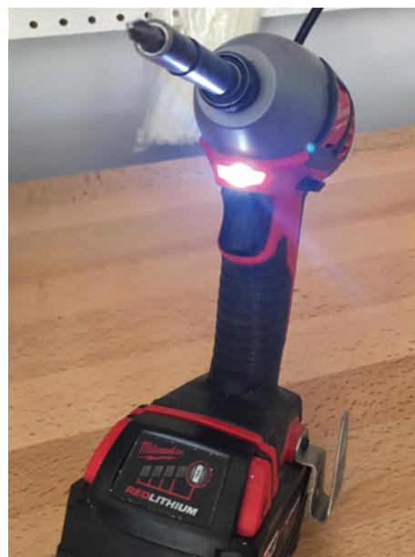
*Figure 5. Cordless 18V impact driver with integrated LED light.*
