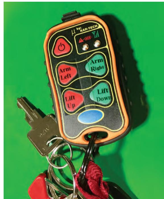
*Figure 10. Wireless controller fob used to position independent and dependent access lifts from lift seat or from another location.*
