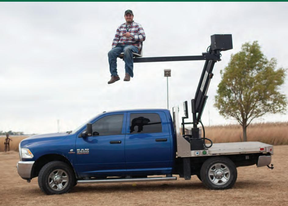
Figure 7. Pickup truck-mounted independent access lift.
