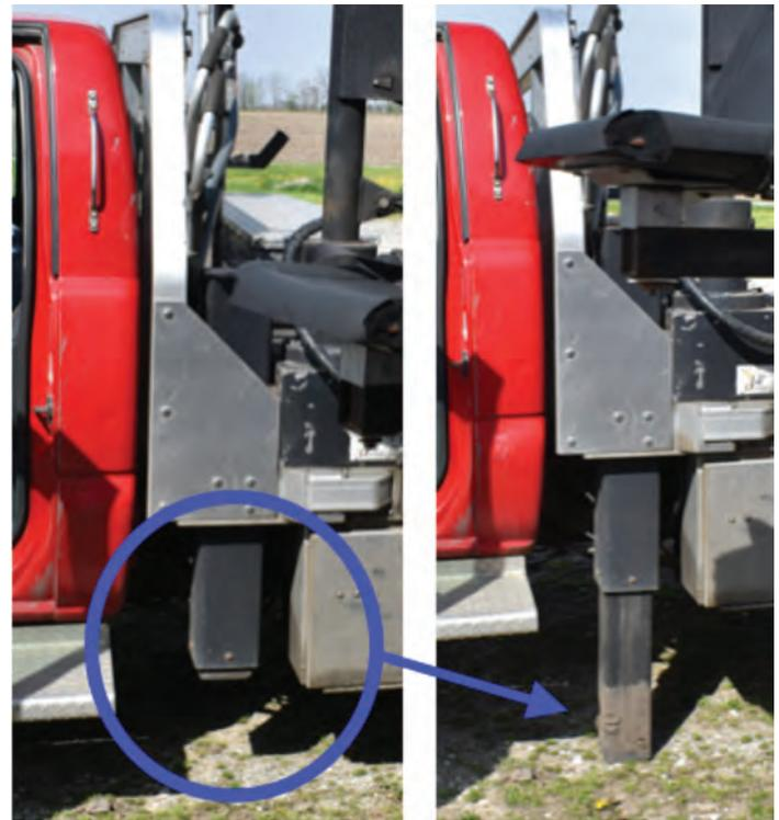
*Figure 11. Stabilizing outrigger on a truck-mounted independent access lift.*
