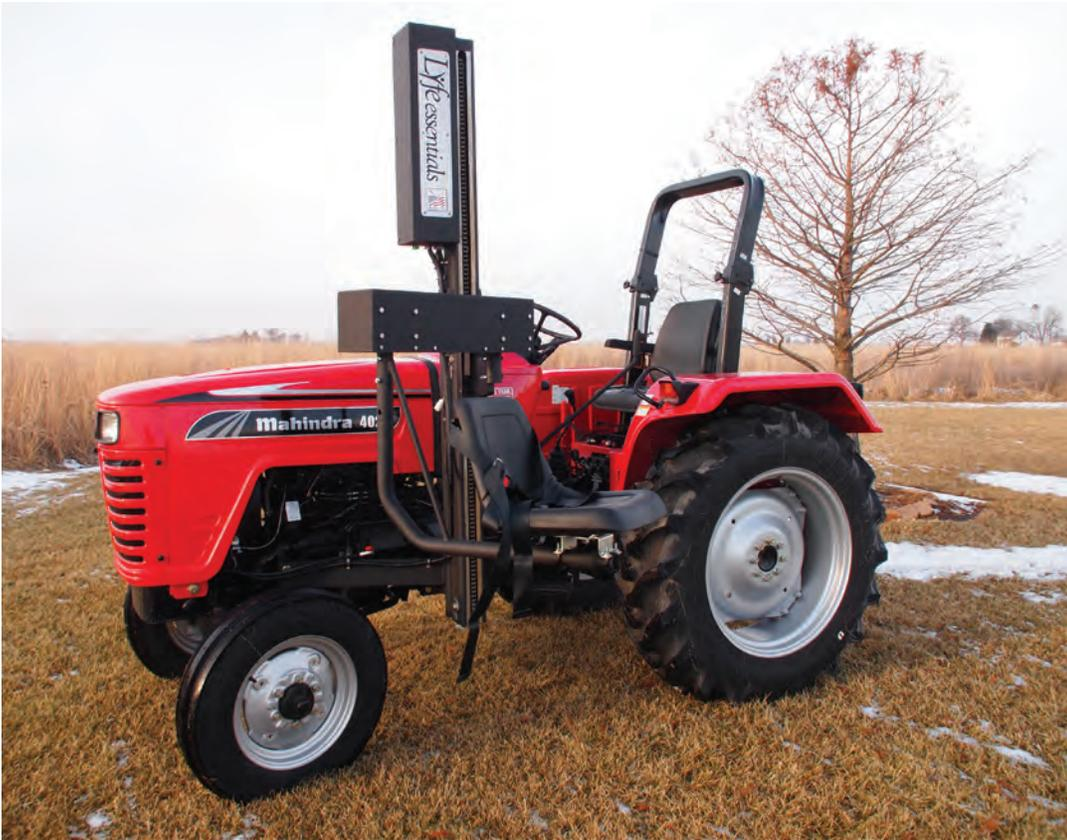
Figure 6. Chair lift mounted to vertical mast. (Source: Life Essentials)
