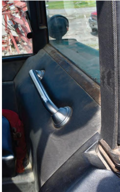
*Figure 12. Additional hand-hold to assist operator in transition to and from access lift seat.*
