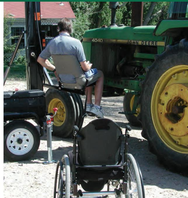
Figure 8. Trailer mounted independent lift.
