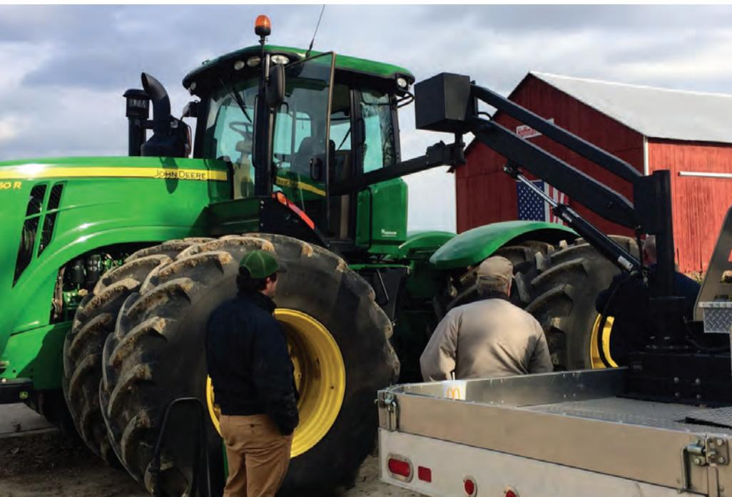
*Figure 9. Independent access lift allows user to access locations up to 12 ft. up and 14 ft. away from the host vehicle.*
