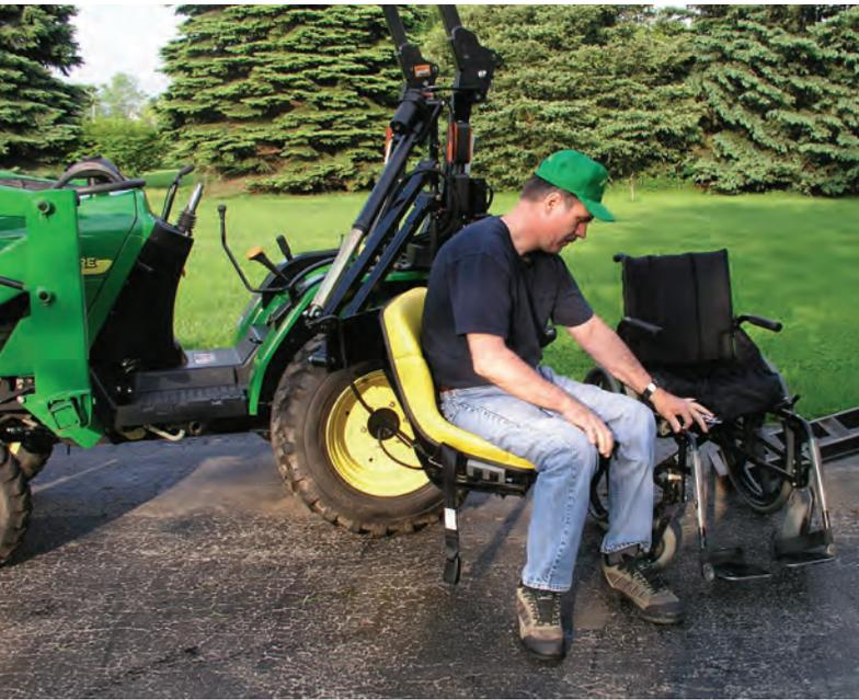
Figure 2. Lift seat doubles as operator seat of tractor, eliminating the need for a second transfer. (Source: Life Essentials)
