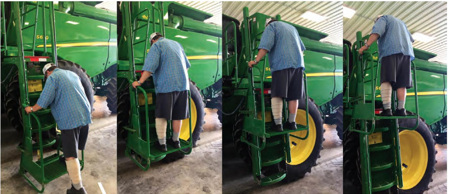
*Figure 4. Platform lift with fold-away platform allows easy entry for both users in need of assistance and able-bodied users.*
