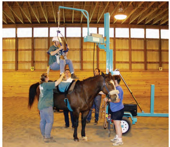
Figure 3. Sling lift used to assist user for horseback riding. (Source: Life Essentials)
