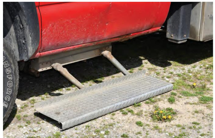
*Figure 5. Running board lift to assist driver (and/or passenger) into vehicle.*
