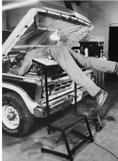
Back-Saver provides a secure object to lean against and adjusts to enable working in awkward positions.
