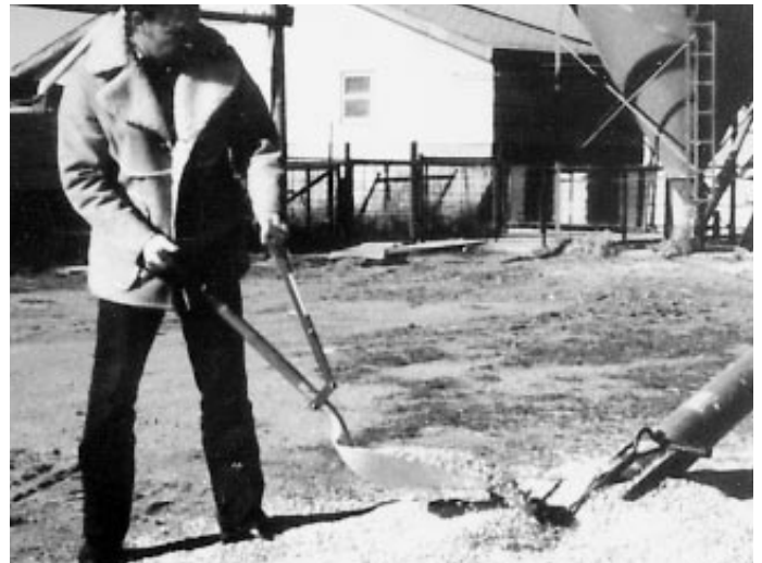
The Scoop-Eeze handle allows the user to stand in a more upright position, reducing back strain.
