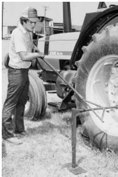
The E-Z Wrench removes and tightens stubborn lug nuts with less stress on the back and joints.
