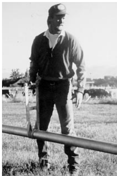
Rick uses a long-handled clamp to grasp the irrigation pipe and reduce the stress on his back.
