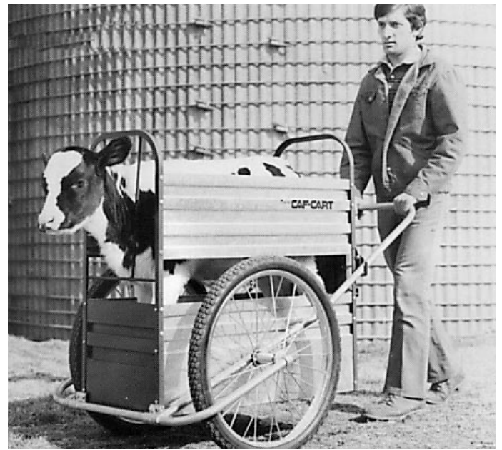
Caf-Cart made with a counter balance axel and ball bearing wheels help reduce back strain.
