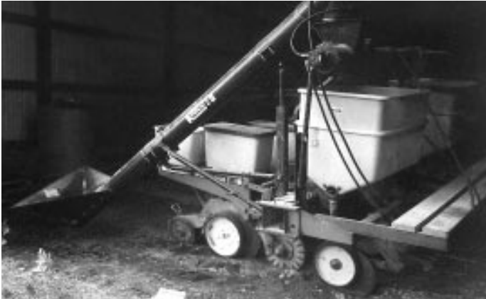
A vertical auger was mounted on the planter to enable fertilizer to be loaded with minimal effort.
