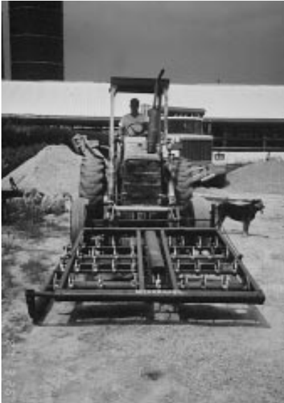
Dennis Herr uses a bale fork attachment to handle hay and avoid further injury to his back.
