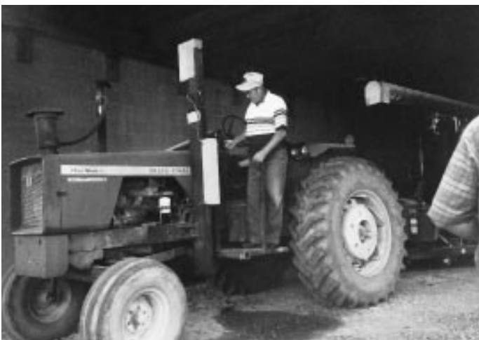
Charlie utilizes a platform lift to access his tractor.
