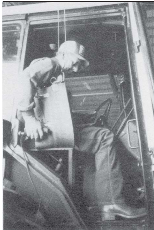
Figure 4. A widely used approach for gaining access to the tractor has been a sling and manually operated hoist.
