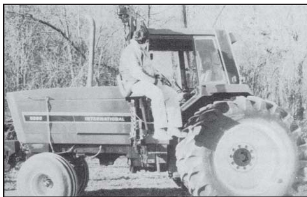
Figure 6. Vertical chair lift manufactured by Simplicity Lifts of West Lafayette, Indiana.
