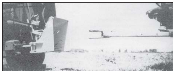
Figure 8. A variety of hitching devices have been introduced which reduce the need to manually hitch trailing implements.
