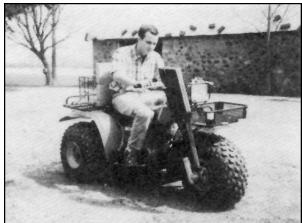
Figure 9. Foam rubber backrest with wire basket support.
