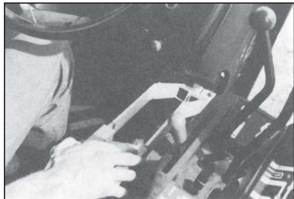
Figure 15. Hand brakes should be constructed to allow for independent or equalized braking.
