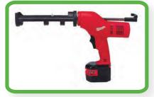
**Cordless Caulk/Adhesive Gun.** Designed to eliminate hand fatigue, this 12-volt lithium-ion, 10-ounce gun reportedly delivers up to 21 inches per minute of caulk or adhesives with 950 pounds of force. Features include a six-setting speed dial, variable-speed trigger, and rotating collar that allows for smooth application around corners. (Visit www.milwaukeetool.com)
