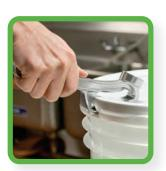
**Plastic-Bucket Lid Opener.** Provides the leverage needed to pry open a 4- to 6-gallon plastic bucket without having to slit or otherwise damage the lid. Works by affixing the opener's "claw" on the rim of the lid and then lifting the handle upward at a couple locations around the lid. Some makes have a hammer-like projection to reseal. (Many different suppliers, including www.webstaurantstore.com.)
