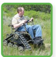
The joystick-operated *Action TrackChair* runs off two 12-volt batteries that feed its 24:1-ratio high-thrust motor. It reportedly has a 5-mph top speed, an 8-mile range, a zero turning radius, and 200-pound load capacity. Standard features include 23-inch-wide seat with 20° tilt, adjustable foot rest, and six accessory holders. Visit www.actiontrackchair.com.
