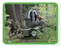
Powered by two 12-volt gel batteries that drive its four motors, the *Journeyman Scooter* is designed to climb hills, cover rough terrain, and wade through up to 6 inches of water without danger of hanging up, tipping over, or stalling out. It features front suspension, large tires, rust-resistant aluminum body, and 4-inch ground clearance. Visit **www.lifeessentiallifts.com**.
