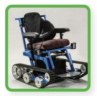
In addition to its outdoor-navigation capabilities (e.g., snow, mud, sand, gravel, grass, even curbs), the joystick-steered *TrackMaster Power Chair*
