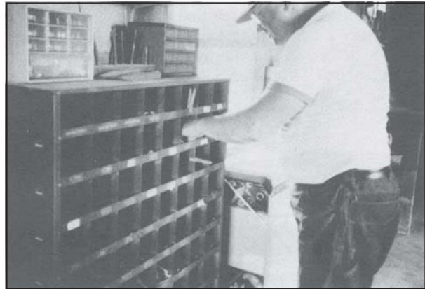
Figure 7. Clothespins help indicate where to return extra nuts and bolts.
